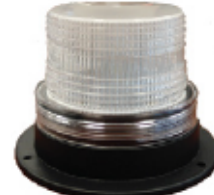
Part No. PRXE-330W Colour White LED 30 diodes Surface Mount with Lead Wires, 3 Mounting Holes @ 4-3/4" diameter
