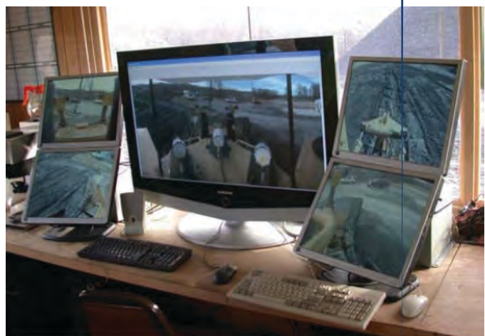
Operator is able to monitor each camera view, independently, on one of four large screens, allowing for safe efficient production. Actual photos from PROVIX IP cameras at Kinross.
