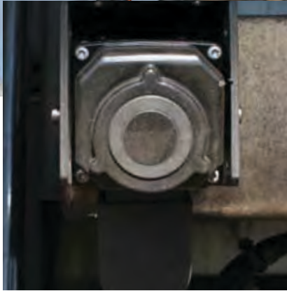
The PathFindIR thermal imaging camera can easily be mounted on front of a mining truck.
