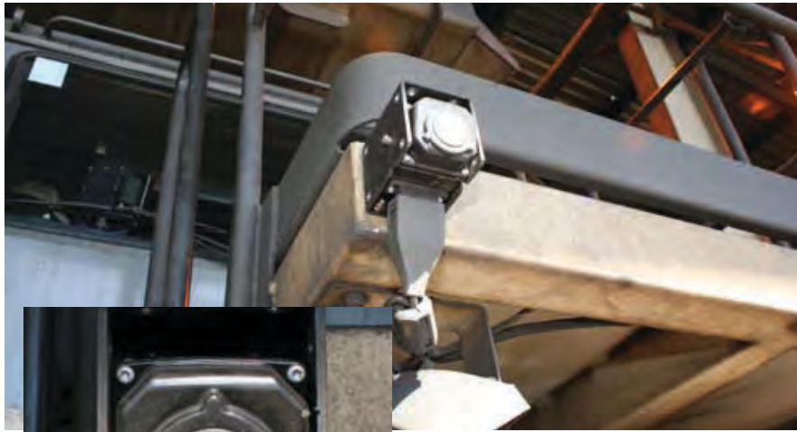
The PathFindIR thermal imaging camera can easily be mounted on front of a mining truck.
