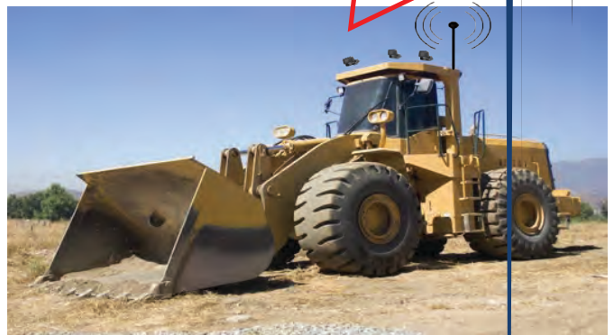
Four PROVIX IP cameras on one of three loaders being run on teleremote by one operator at Fort Knox- Kinross Gold Alaska.
