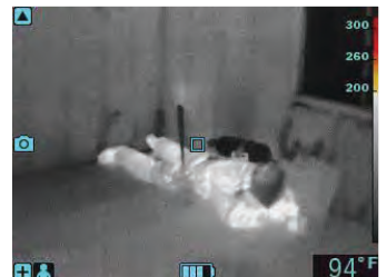
For use with lower temperature situations, such as initial rescue efforts after traffic accidents, searches in wooded landscapes, etc.
