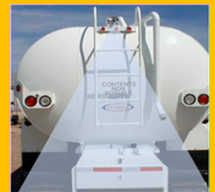
Explosion proof camera on the back of a Tanker truck
